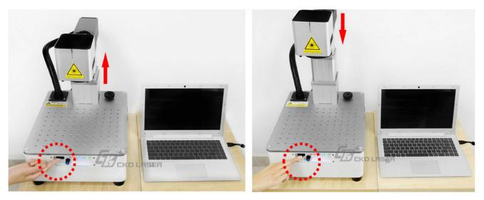
Dial this switch upward, the marking head goesup, dial it downward, the marking head goes down, the next speed knob is usedfor adjusting the move speed, so that the focusing adjustment can be fast orslow down precisely.
