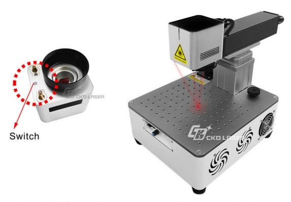
It's right focus when three red dots overlap. There are two dots fixed under the galvanometer, so that they are not easy tobe disturbed during and avoided off-set. The switch under the galvanometer controlthose two lights on/ off to expand service life or avoiding distraction when engraving special material. Easy change from outside for those lights, avoiding open thelaser to replace or maintenance.
